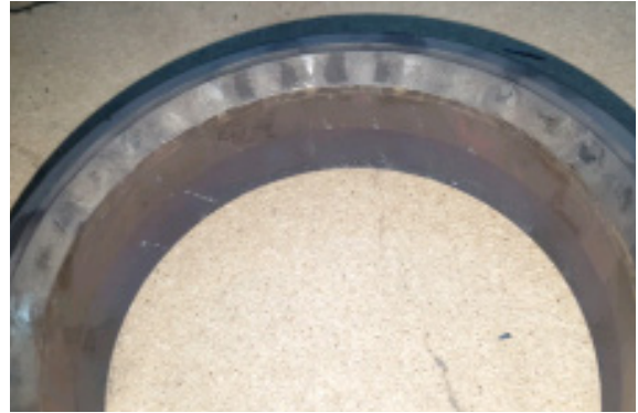
High velocity jets have caused erosion damage on a valve seat, with leakage as a result.
