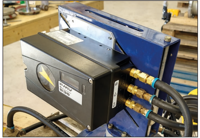
D30 POSITIONER RETROFITTED TO STI ACTUATOR
